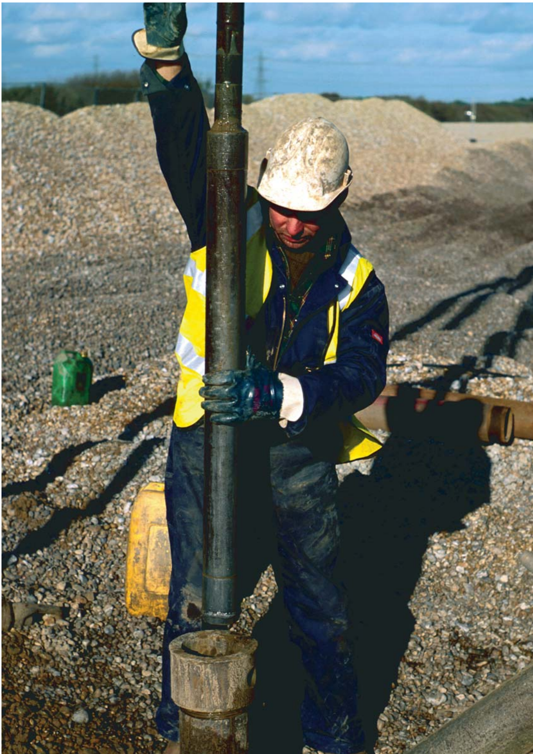
The percussion drilling rig used in the Dungeness and Port of Rye projects collecting sediment from close to Dungeness Power Station
