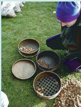
Sieving different grain size fractions from the deep Dungeness cores.
