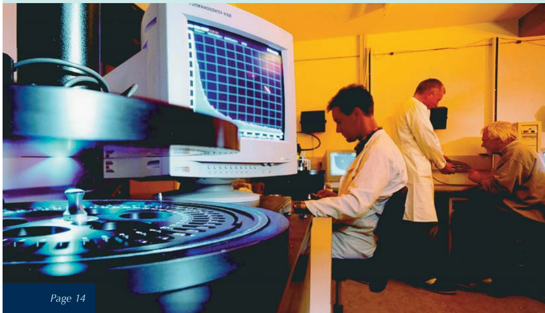
A Risø reader used for laboratory-based luminescence measurements
