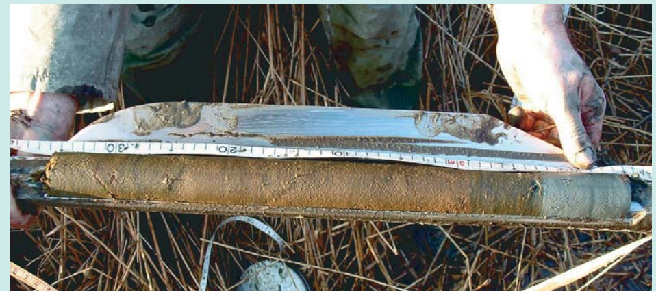
Sample core collected from the middle of Muddymore Pit. In the base of the core are grey silty sands that accumulated under marine tidal conditions. These sediments pass upwards into a largely freshwater organic mud
