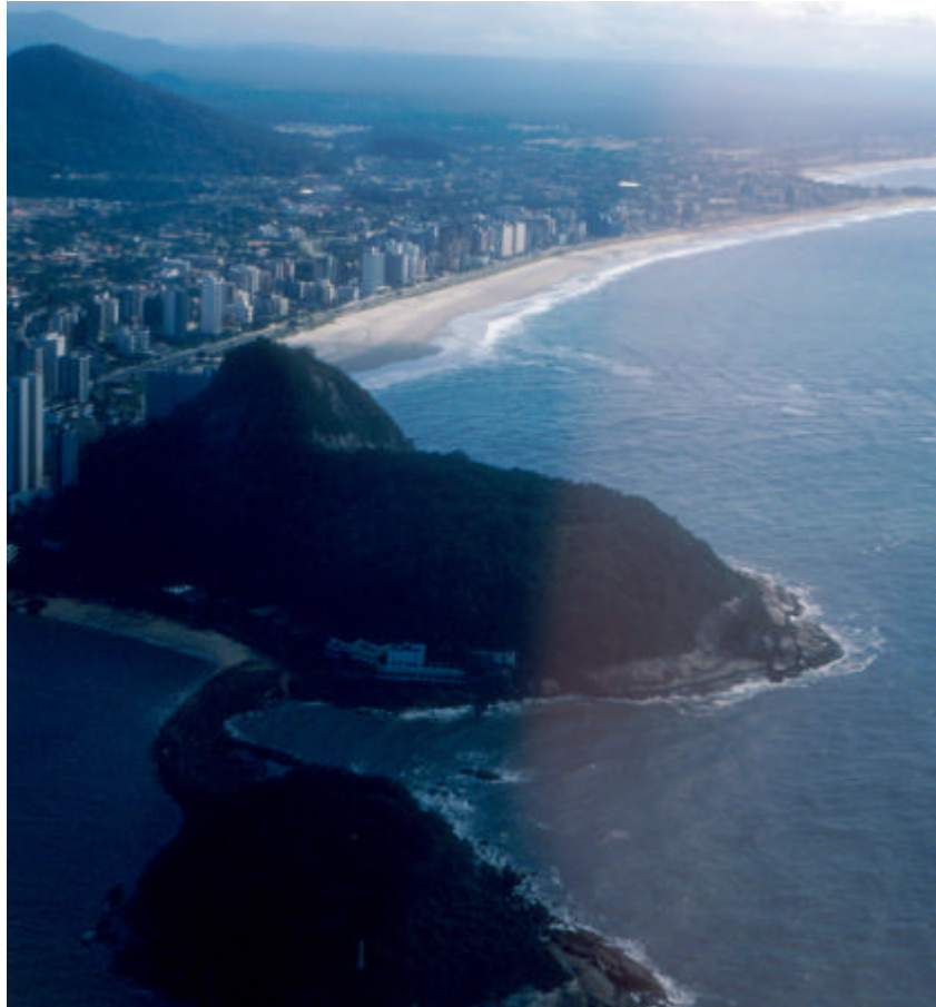
Figure 10: Caiobá hill and Caiobá beach. Note the beach enlargement and the wave refraction pattern induced by the ebb tidal delta lobal front.
