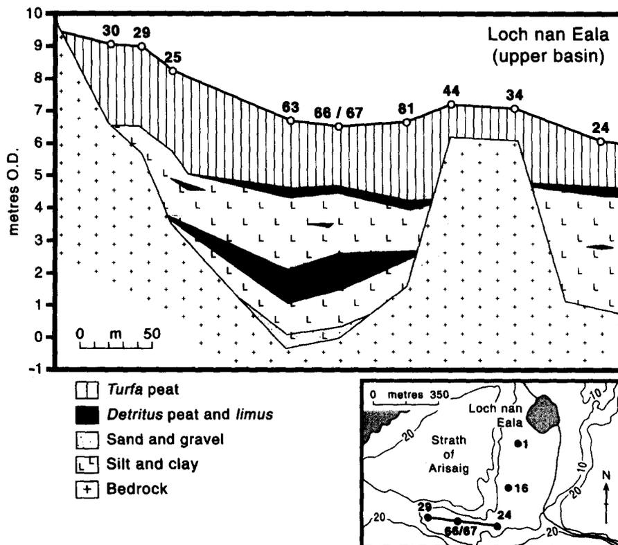
FIG. 5. Location of the borehole transect and generalised stratigraphy in the upper basin at Loch nan Eala. Cores 24, 16 and 1 are in the main basin.
