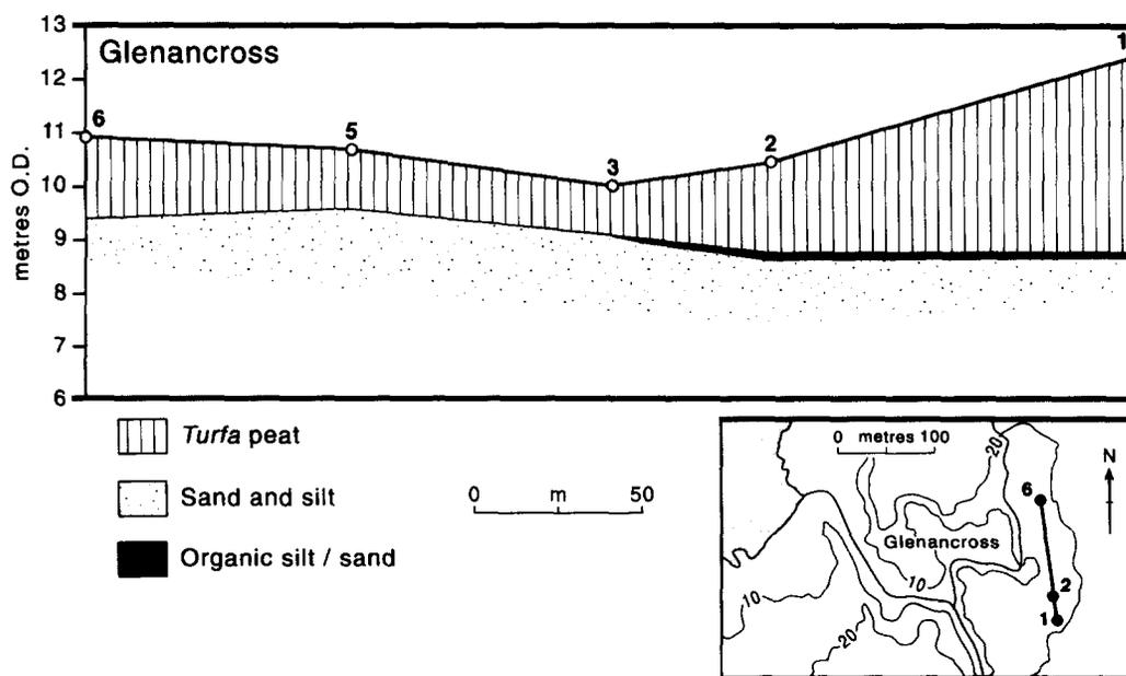
FIG. 11. Location of the borehole transect and generalised stratigraphy at Glenancross.
