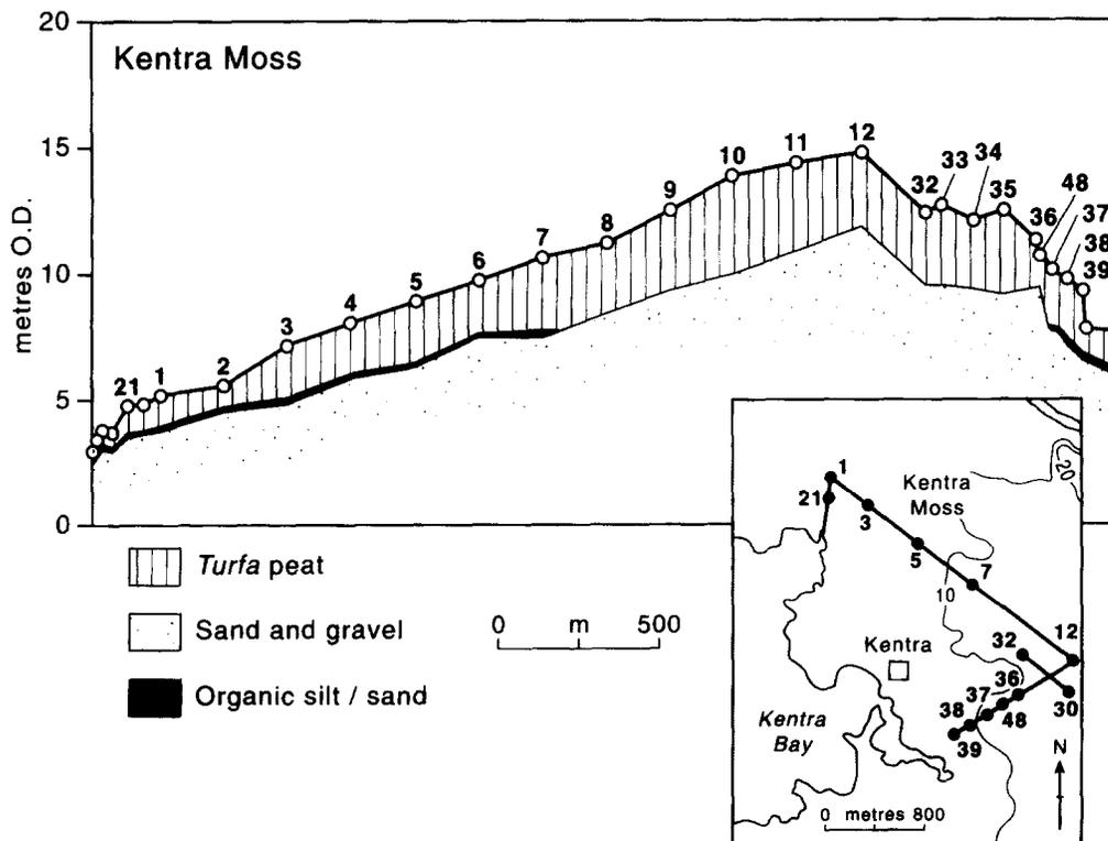
FIG. 3. Location of borehole transects and generalised stratigraphy at Kentra Moss. Stratigraphic symbols in this and all following diagrams are after Troels-Smith (1955) except where modified for clarity of presentation.
